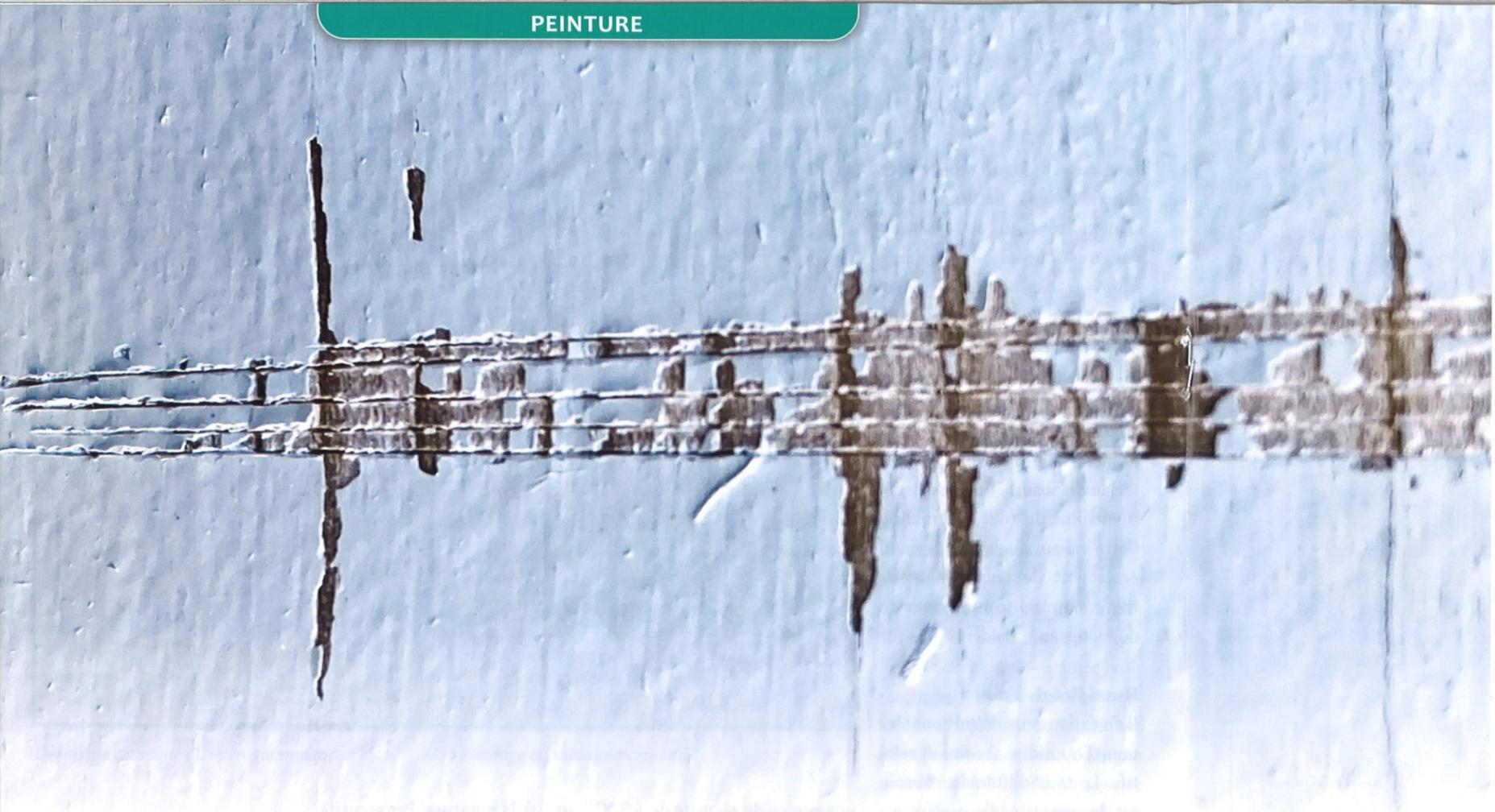
Test de quadrillage
